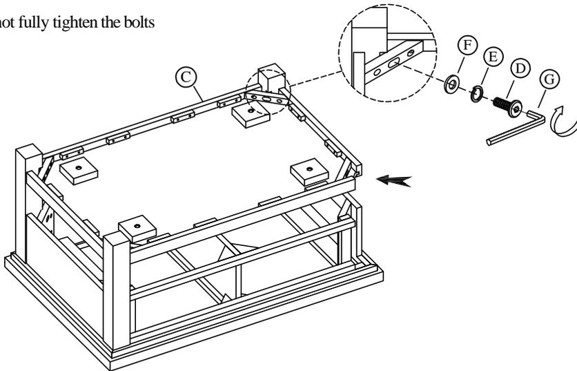
STEP 4: Using the Allen key (G) tighten all bolts
